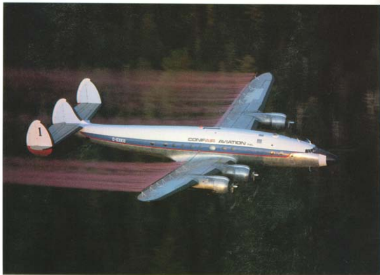
Ideal spraying time for the 'budworm bombers' is when the air is stillest, early morning or evening. Captured from an Aztec chase plane, one of the Connies is seen in action one evening in the region of Matane, Quebec. Its chemical 'cargo' is coloured to aid visual monitoring.
