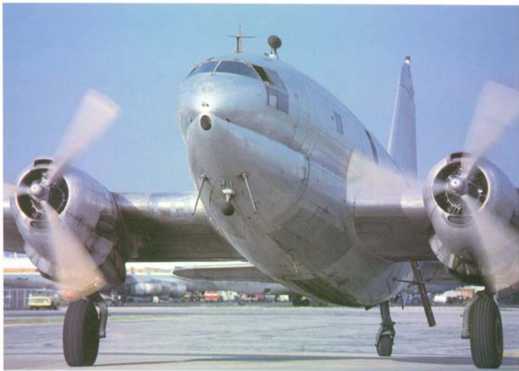
About 100 C-46s remain active. They offer a generous payload and the type remains competitive, although poor single-engine performance has caused many a ditching. This natural metal C-46, N1807M, has changed hands many times, but remains based out of Miami's Corrosion Corner
